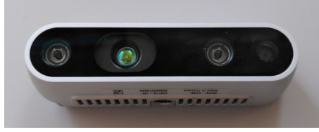
Figure 2.3: The RealSense™ D435i depth camera, with the left IR camera, IR pattern projector, right IR camera, RGB camera
